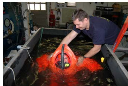
Fig. 1: Buoyancy testing of the MK10 SEIE suit in the immersion tank at NSMRL. After fully inflating the hood the subject was submerged via a pulley system attached to a waist belt until the top of the hood was approximately 4 inches below the water surface. The tension in the pulley system was then slowly released to just overcome pulley friction while forces in the line were measured using a force transducer.
