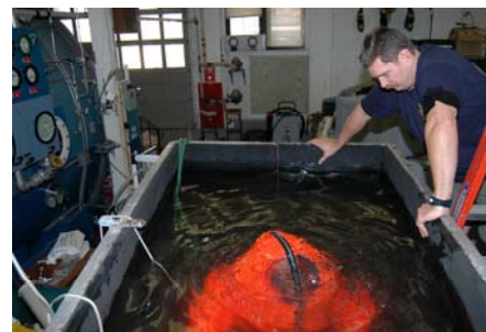
Fig. 1: Buoyancy testing of the MK10 SEIE suit in the immersion tank at NSMRL. After fully inflating the hood the subject was submerged via a pulley system attached to a waist belt until the top of the hood was approximately 4 inches below the water surface. The tension in the pulley system was then slowly released to just overcome pulley friction while forces in the line were measured using a force transducer.
